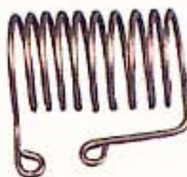
First speed. 9 gauge wire
