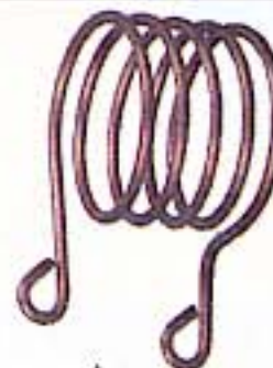
Second speed, 7 gauge wire
