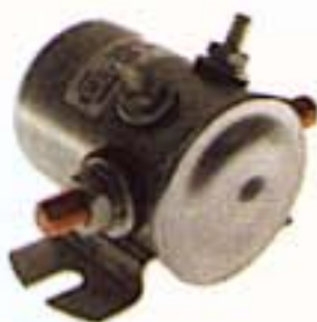
#70 series. 36-volt, 4 terminal with silver contacts. Short housing
