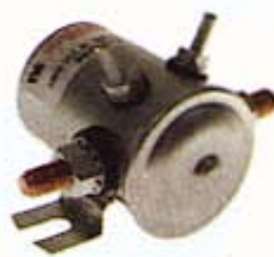
#71 series. 36-volt, 4 terminal with copper contacts. Long housing
