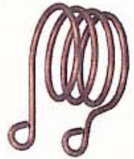
Third speed. 6 gauge wire
